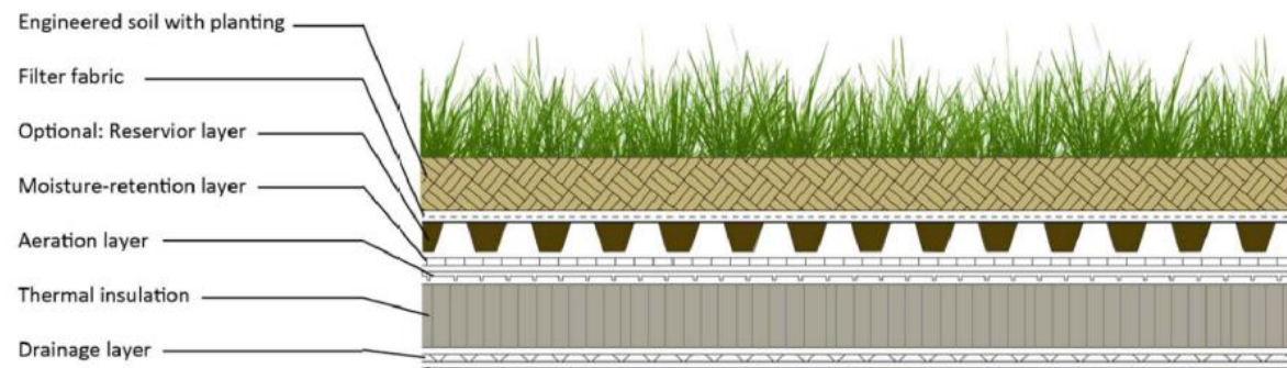
Typical details illustrating the SuDS bio-retention system under the roof garden.
