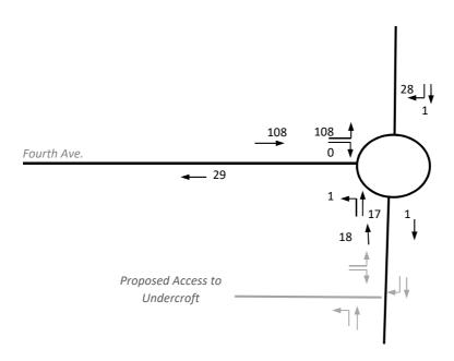
Existing Roundabout to be Upgraded to Signal Control (Refer to Drawings)
