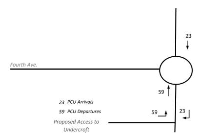
Existing Roundabout to be Upgraded to Signal Control (Refer to Drawings)
