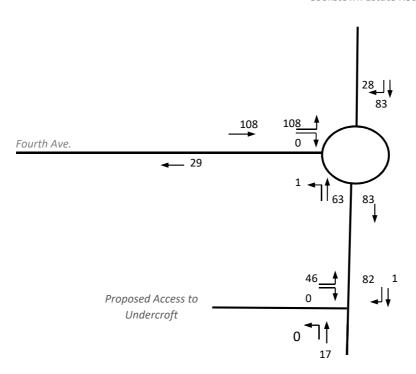
Existing Roundabout to be Upgraded to Signal Control (Refer to Drawings)
