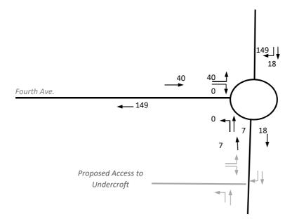
Existing Roundabout to be Upgraded to Signal Control (Refer to Drawings)
