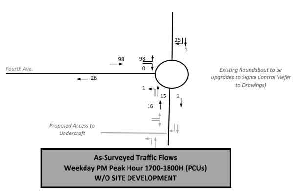
NRA Project Appraisal Guidelines Unit 5.5, Table 5.5.1 National Traffic Growth Forecasts for SDCC, Medium Growth to 2023 factor is 1.035 and then to 2038 factor is 1.104 - These have been used to Factor the Background Traffic to Selected Opening & Design Year Conditions.
