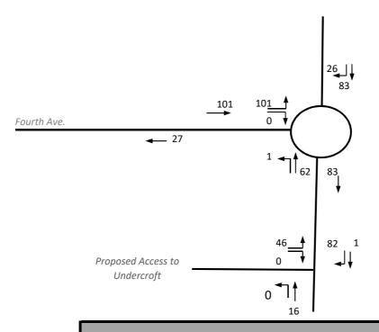
Existing Roundabout to be Upgraded to Signal Control (Refer to Drawings)
